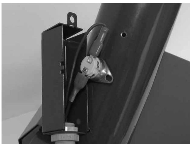
Fig. 10 - Safety thermostat on the pellet supply pipe, 95 °C
