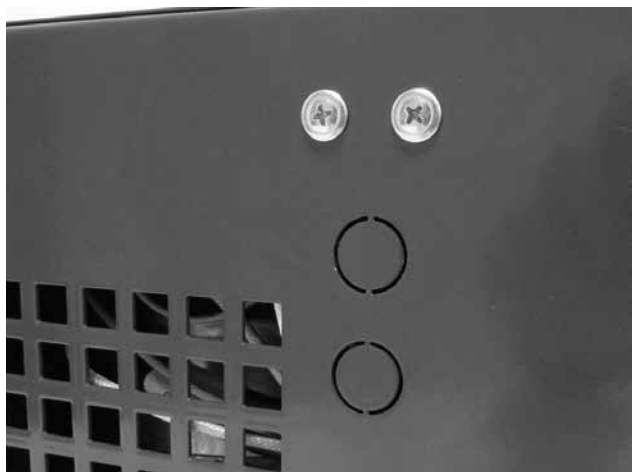
Fig. 11 - – unrifled openings originally for TS and TV temperature sensors (may be used for other applications)
